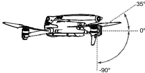
Use the gimbal dial on the remote controller to control the tilt of the camera. Alternatively, enter the camera view in DJI Fly. Press the screen until an adjustment bar appears and drag up and down to control the tilt of the camera.
